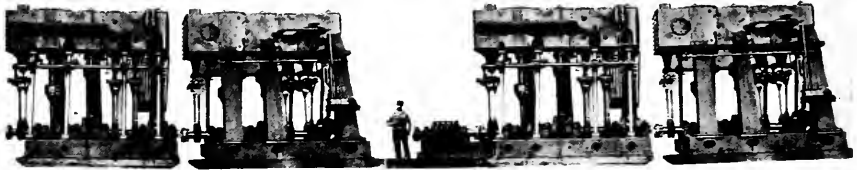
Four triple expansion engines built by the Seattle Machine Works to the order of the Pacific American Fisheries.
